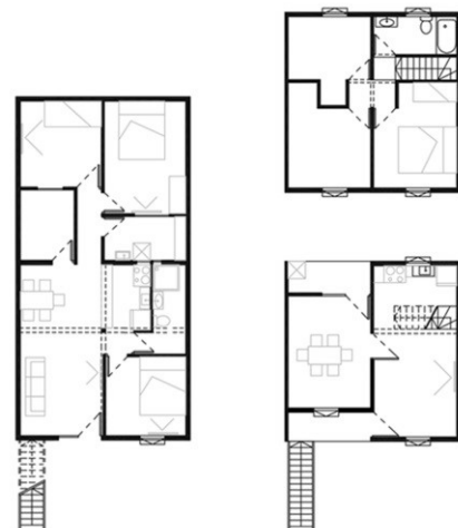
Figure 3. Floor plan of the extended base house of Lo Espejo: (left) first floor house; (right) duplex house (source: the author)
