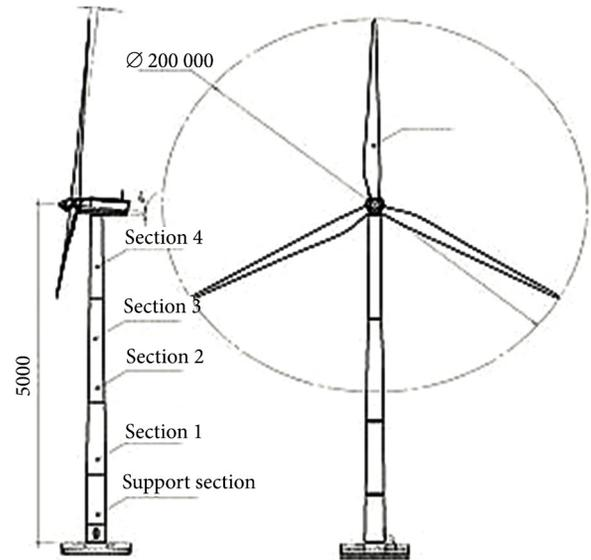
Figure 3. Scheme of a wind turbine
