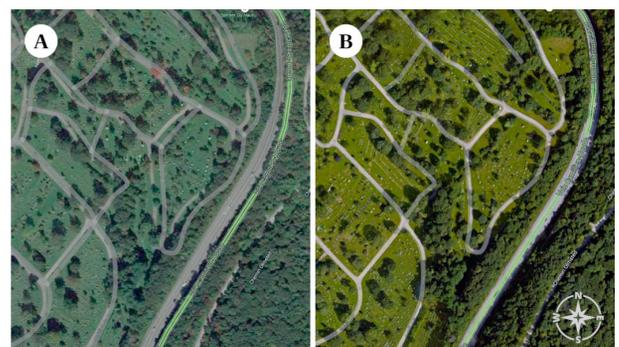
Fig. 4. Relief displacement in Mount Royal, the city of Montreal, (A) before, and (B) after correction. This location is marked by a green square in Fig. 1
