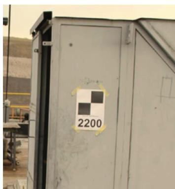
Fig. 3. Control point marks for ScanStation C10 and for Faro Focus 3D
