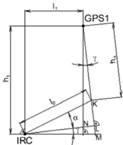
Fig. 7. Inclined bucket-wheel excavator with bucket wheel below IRC plane ( $|\gamma| < |\beta|$ ) and IRC joint detail image
