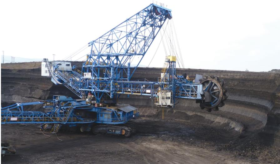
Fig. 1. Bucket-wheel excavator K800/N1/103
