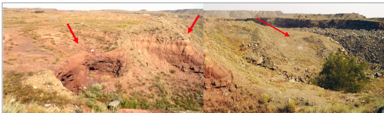
Figure 4. Dips over mine voids (near the t. Rudnik, Zhezkazgan ore field). The arrows indicate the places of dips
