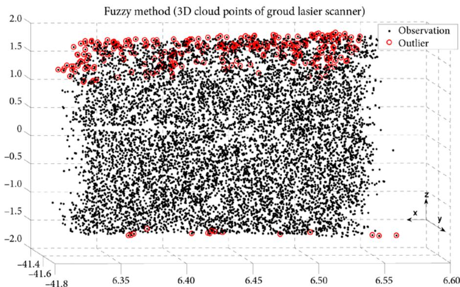
Fig. 3. Outliers detection based on Fuzzy approach applied into the 3D point clouds of the ground-based laser scanner ( $x$ ,  $y$  and  $z$  [m] are assumed in a local coordinate system).
