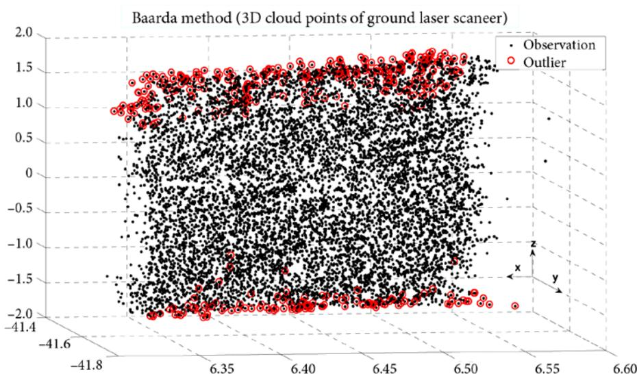
Fig. 2. Outliers detection based on Baarda method applied into the 3D point clouds of the ground-based laser scanner ( $x$ ,  $y$  and  $z$  [m] are assumed in a local coordinate system).
