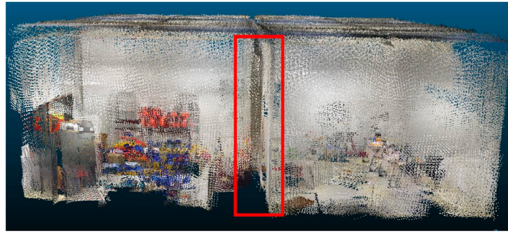
Figure 6. Void areas in the 3D point cloud model (Red Box)
