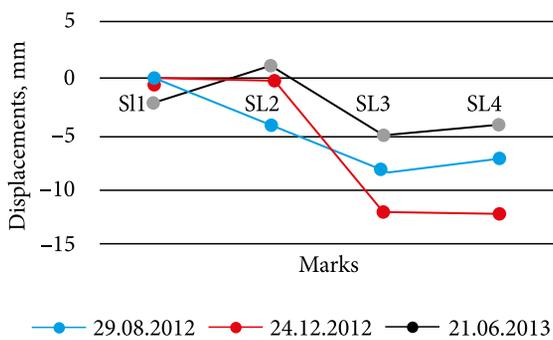
Fig. 5. The displacements of the reflectors in the direction of the cross axis for the south-east facade
