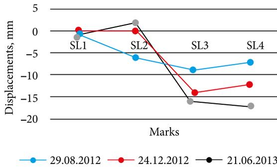
Fig. 4. The displacements of the reflectors in the direction of the cross axis for the north-east facade.
