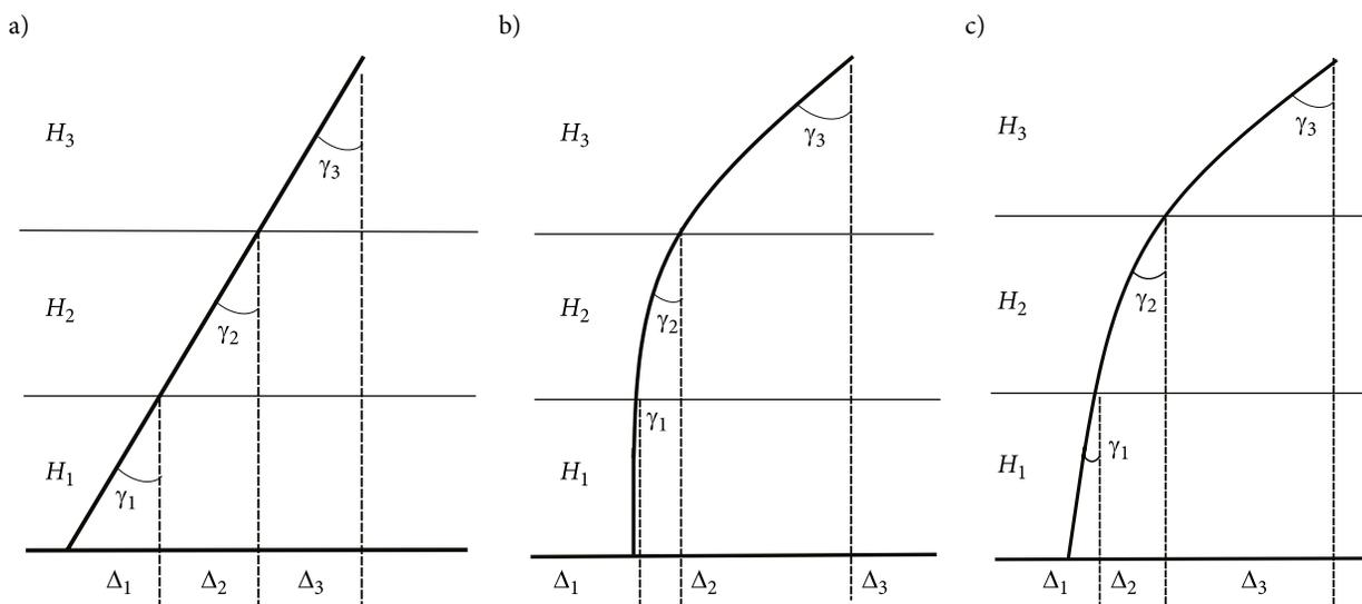
Fig. 1(a). Variants of axis displacement of the building – building pure roll (displacement)
