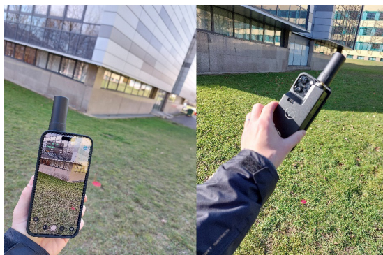
Figure 5. Measuring process in the field with viDoc RTK rover
