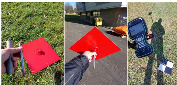
Figure 4. Ground control points – technical solution and GNSS measurements
