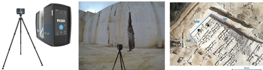
Figure 5. FARO Laser Scanner S70 (left); equipment during data acquisition (center); the façades viewed over a base map from Google Maps ( google.com/maps )
