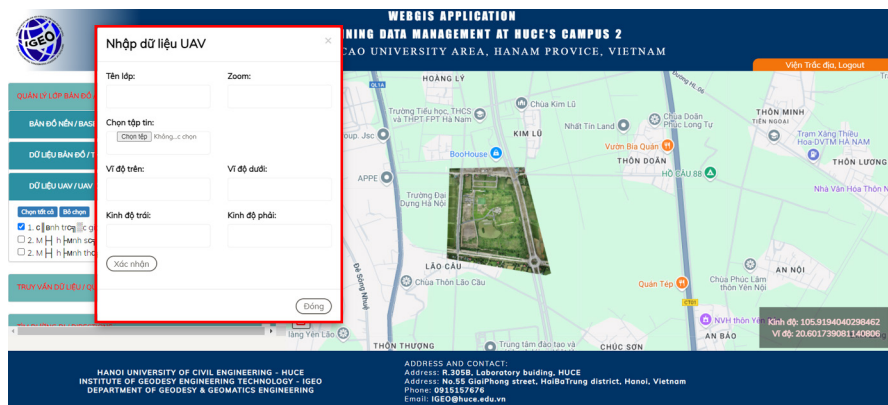
Figure 7. Direct importation of orthomosaic data devired from UAV data into the WebGIS system
