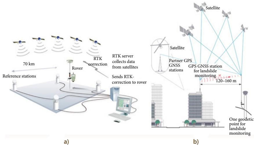
**Figure 3.** The operation principle of the network of permanently operating satellite base stations (a) and the station at the research object (b)
