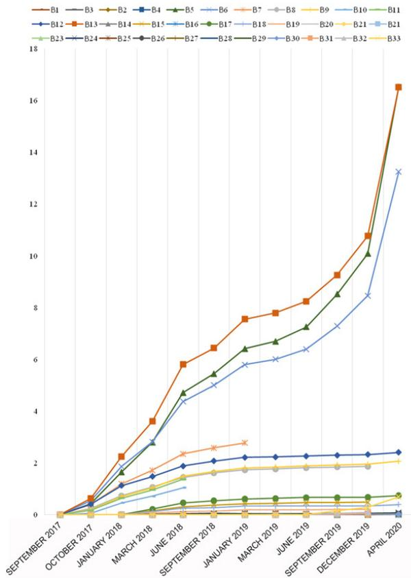
**Figure 7.** Graphic display of quarterly absolute deviation of ground benchmarks (formed based on the results of own research)
