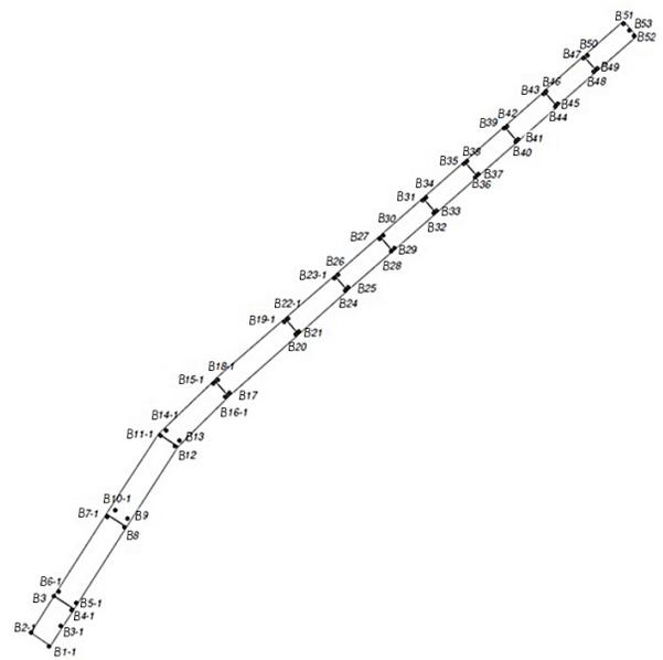
**Figure 8.** Scheme of geodetic benchmarks laid on the coastal fortification structure
