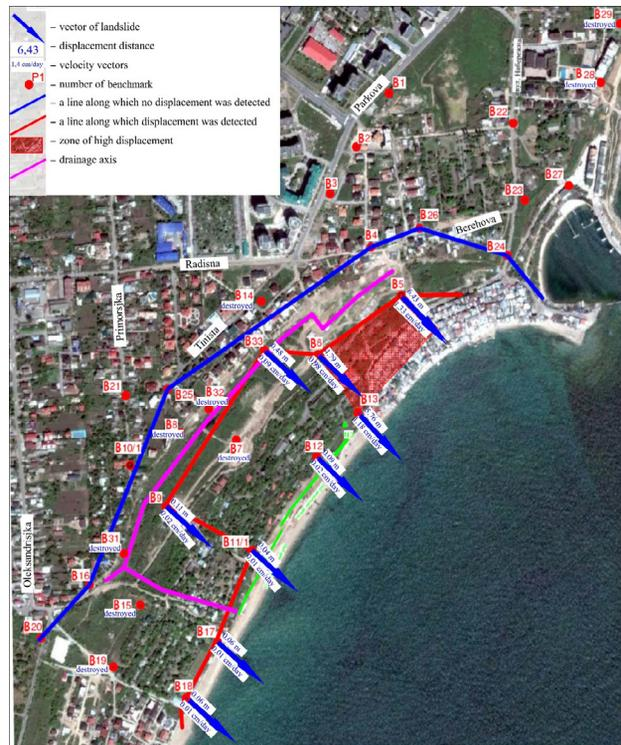
**Figure 6.** Displacement and velocity vectors of benchmarks with their display on the map from September 2017 to April 2020
