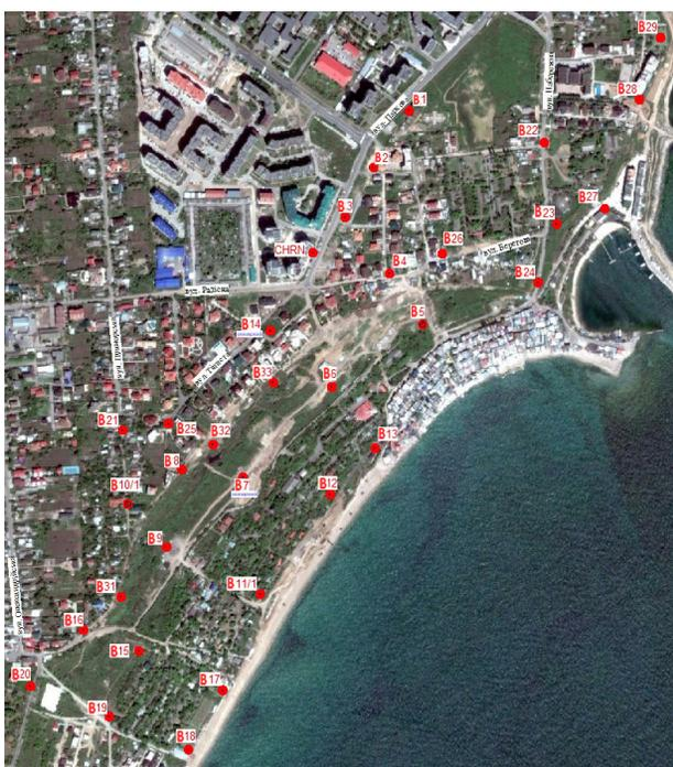
**Figure 4.** The scheme of laid ground benchmarks (based on Google Maps, n.d.)
