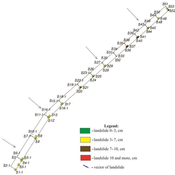
**Figure 9.** Displacement vectors and a quantitative indicator of the displacement of benchmarks on the coastal fortification structure for the last observation period
