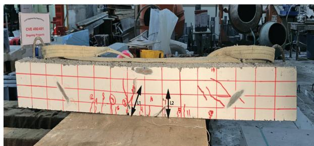
**Figure 3.** Experimental setup of Mix#2 with defined cracks
