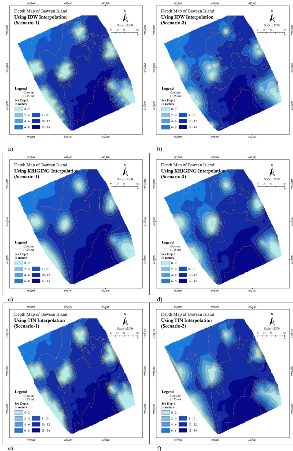
Figure 3. Depth map generation using the first scenario (left) and second scenario (right): a – IDW first scenario; b – IDW second scenario; c – Kriging first scenario; d – Kriging second scenario; e – TIN first scenario; f – TIN second scenario
