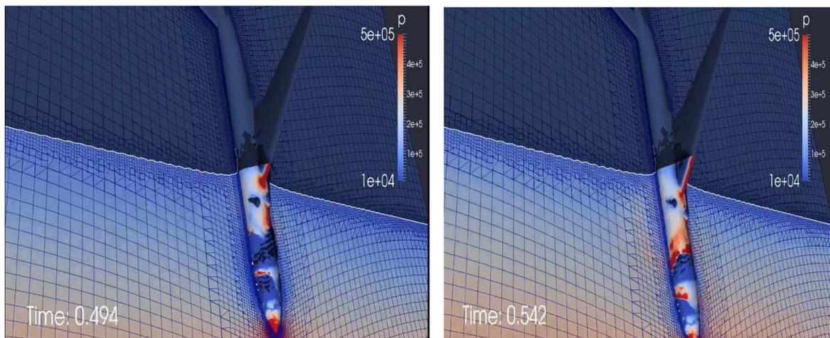
Figure 11. This is a nose-dive situation (Pitch angle =  $-90^\circ$ , angle of approach =  $93^\circ$ ) of MH370 (Chen et al., 2015)
