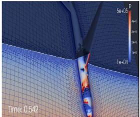
Figure 11. This is a nose-dive situation (Pitch angle  $= -90^{\circ}$ , angle of approach  $= 93^{\circ}$ ) of MH370 (Chen et al., 2015)
