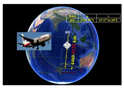
Figure 4. Maximum (red circle) and minimum (yellow circle) distance values that the aircraft (MH370) will travel from the second arc (K0 point) according to fuel condition and consumption
