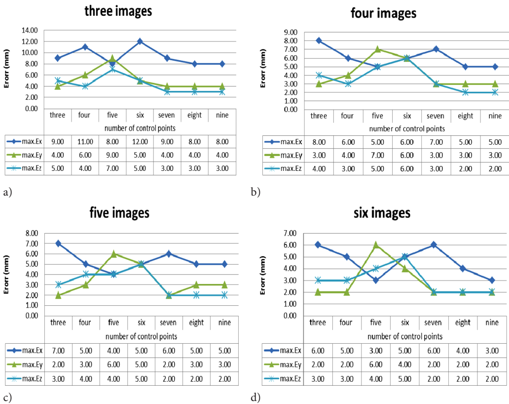
Figure 9. Effect of ground control point's numbers on maximum point coordinates differences between total station observations and metric camera with photogrammetry scanner
