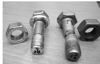
Figure 3. Fracture modes of the non-preloaded regular bolts (on the left) and high strength bolts (on the right)
