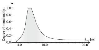
Fig. 13. Fuzzy buckling length of the left column
