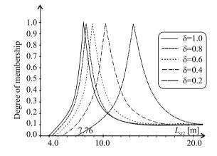
Fig. 9. Fuzzy buckling length of the right column
