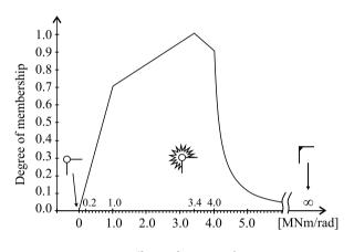
Fig. 5. Stiffness of semi-rigid joints
