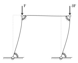
Fig. 2. Buckling a frame with a semi-rigid joint
