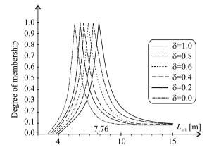
Fig. 8. Fuzzy buckling length of the left column
