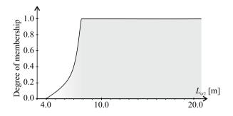
Fig. 11. Fuzzy buckling length of the right column
