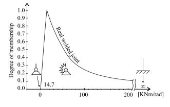
Fig. 3. Stiffness of support joints
