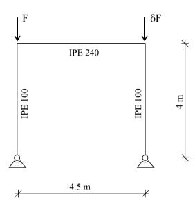
Fig. 1. The geometry of a steel plane frame
