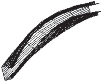
Fig. 21. The global flexural buckling mode (FTM) of Rack column
