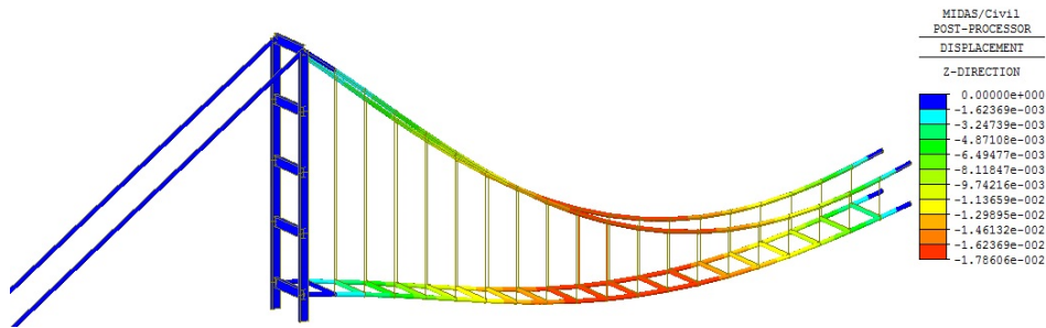
Figure 5. A deformed finite element model for the bridge under symmetrical loading ( \xi = 1.0, \gamma = 1 )
