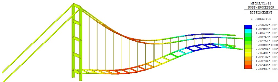
Figure 10. A deformed finite element model for the bridge under asymmetrical loading ( \xi = 1.0, \gamma = 1 )
