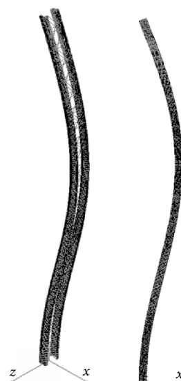
Fig. 6. The mode of the flexural buckling shape of the steel built-up column about axis z-z (out-of-plane)
