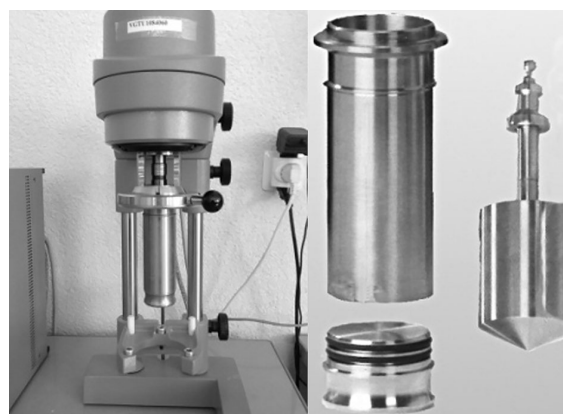
Fig. 2. Illustration of the rheometer used (shown with coaxial cylinders)
