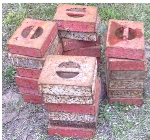
Fig. 6. 30 kPa surcharge around dynamic plate
