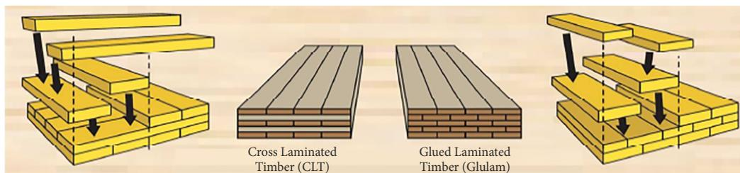
Figure 1. Difference between CLT and glulam (Avellan, 2018)
