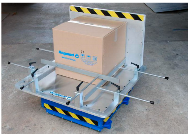
Figure 2. Laboratory shaker for testing damage to packaging with contents in the transport process (source: own development)
