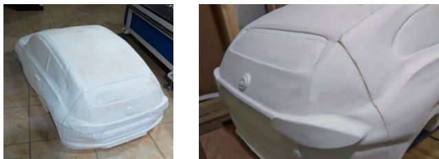
Figure 8. Scaled prototype of an electric vehicle concept, fabricated using computer-aided design routing of expanded polystyrene foam from a digital three-dimensional computer numerical control model prepared by the student who participated in the study (source: created by Sherief Fawzy, fabricated by Creative Solutions Factory )
