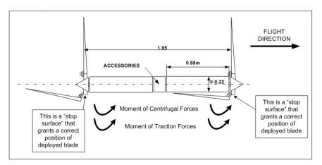
Fig. 9. Propellers with folding blades: similar solutions for puller and pusher propellers
