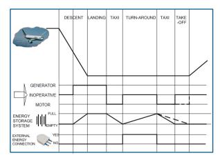
Fig. 11. Hybrid propulsion system operation cycle from the aircraft's descent to take-off
