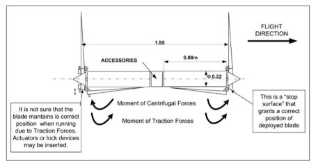
Fig. 8. Propellers with folding blades: different solutions for puller and pusher propellers
