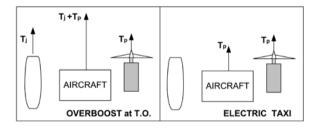
Fig. 1. Hybrid propulsion scheme for jet propelled aircraft
