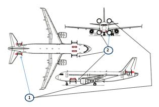
Fig. 10. Two solutions of the hybrid propulsion system installation
