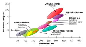
Fig. 4. Volume and weight for several type of energy storage systems
