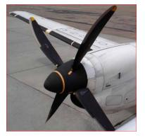
Fig. 6. Propeller in a feathered position
