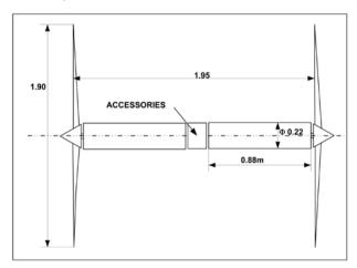
Fig. 5. Two propellers and electric motor-generators in a tandem configuration
