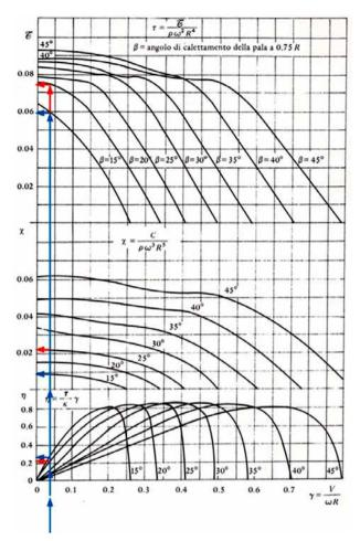
Fig. 3. Propeller Plots (NACA four-blades). From (Lausetti 1992)
