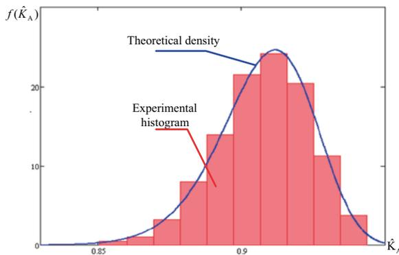
Fig. 4. PDF and histogram of the ready-to-operate factor estimation for the case of exponential distribution of the operating time between failures and recovery time
