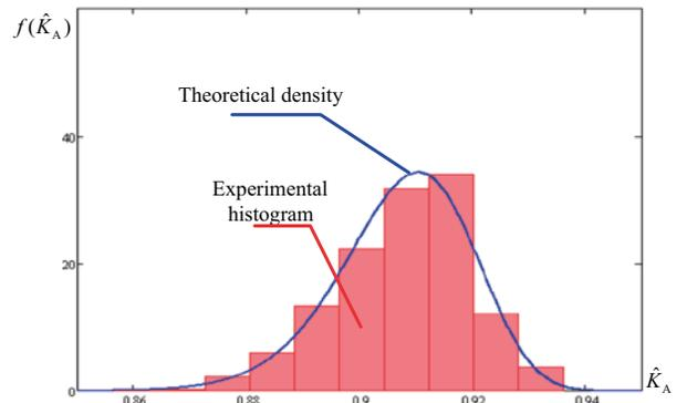
Fig. 5. PDF and histogram of the ready-to-operate factor estimation for the case of exponential distribution of the mean operating time between failures and a stable recovery time
