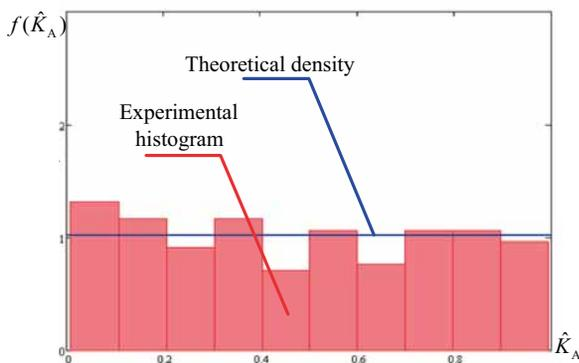
Fig. 8. PDF and histogram of the ready-to-operate factor estimation for the case  $T_0 = T_R$  and  $n = 1$
