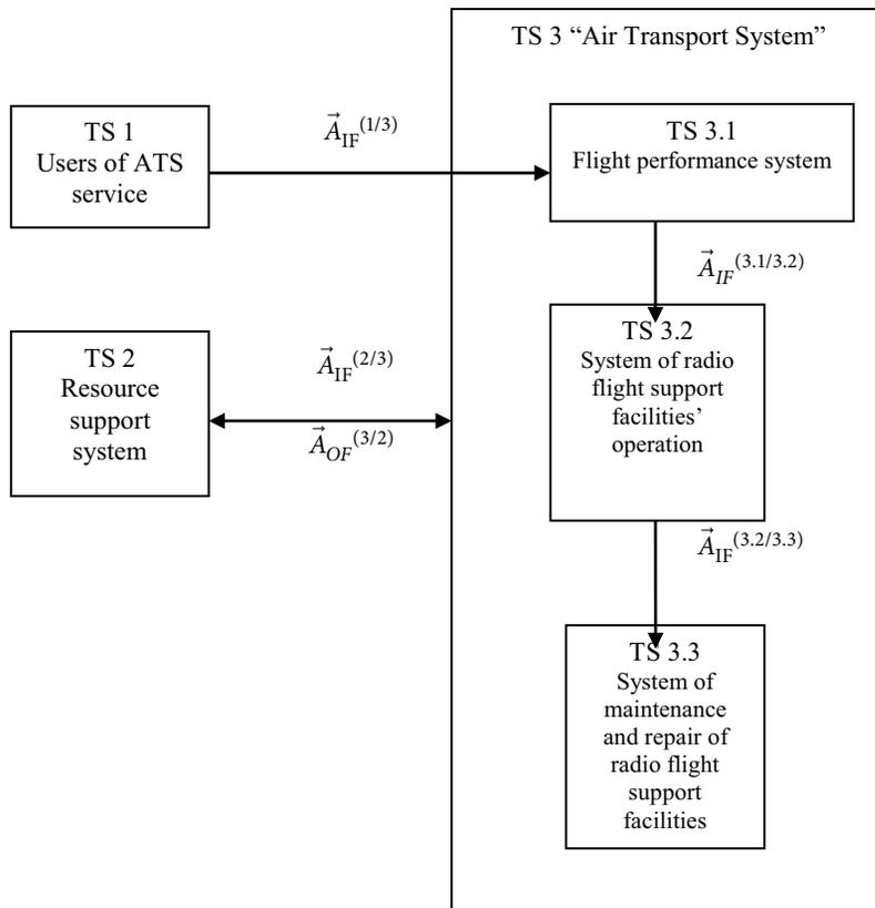
Fig. 1. Generalized structural diagram of the interaction between the technological systems in the ATS
