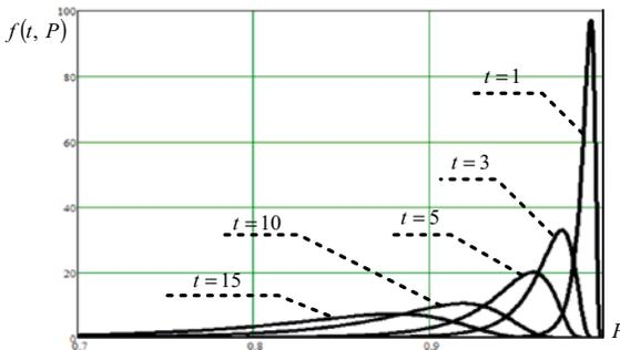
Fig. 3. Nomograms for the PDF of no failure operation in a finite time interval
