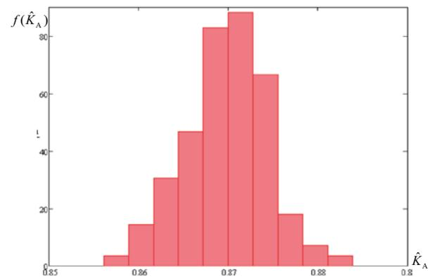
Fig. 6. Histogram of the ready-to-operate factor estimation for the case of normal distribution of operating time between failures and recovery time
