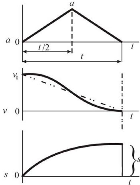
**Fig 6.** Rate of deceleration with a symmetrical triangular form
