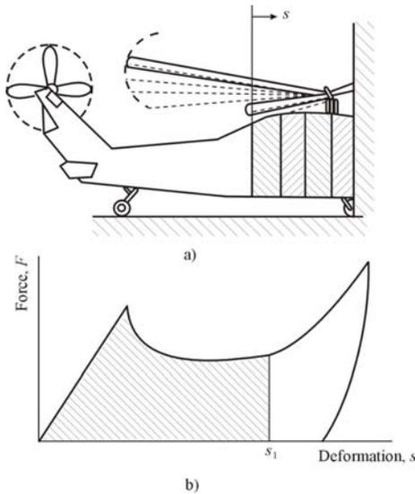
**Fig 1.** Kinetic energy descending during impact
