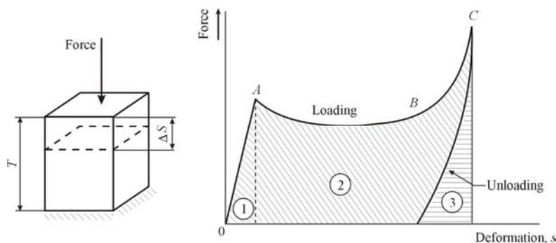
**Fig 2.** Force and shift interdependence of porous composite
