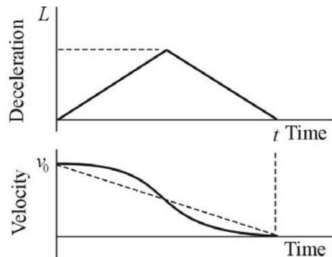
**Fig 9.** Rate of deceleration with a triangular form (No 2)
