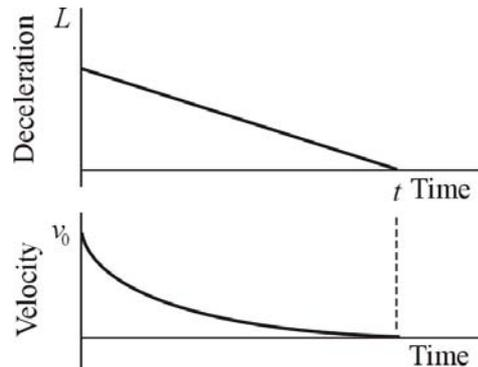
**Fig 8.** Rate of deceleration with a triangular form (No 1)
