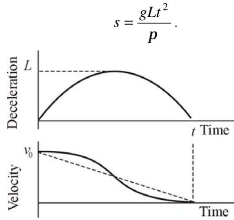
Fig 11. Rate of deceleration with a half-sine form
