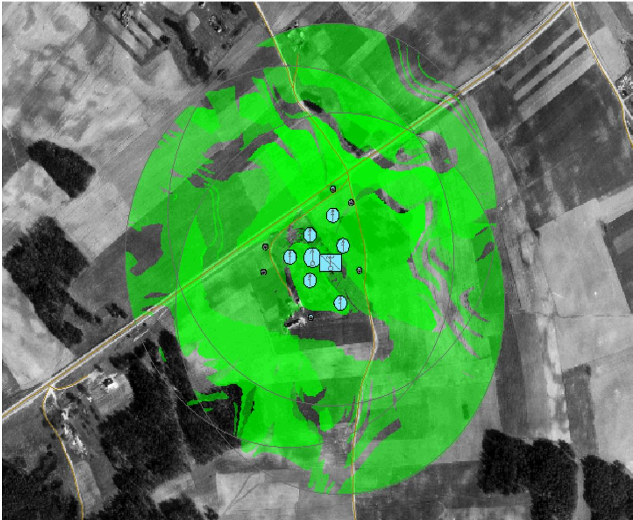
**Fig 3.** A combined analysis of the visibility for gunners in the angles (radius of visibility – 300 m, sighting point height – 2 m, height of the objects to be observed – 0 m) maintaining the scheme of the ambush and graphic basis of the terrain
