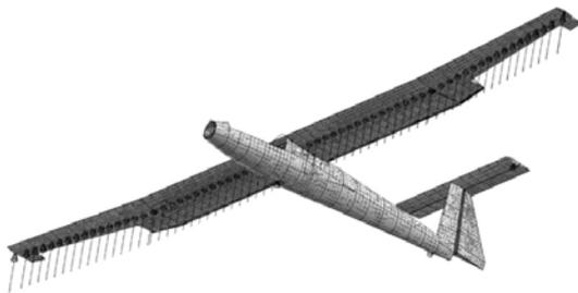
Fig 9. Forces and constrains simulating symmetrical steady flight
