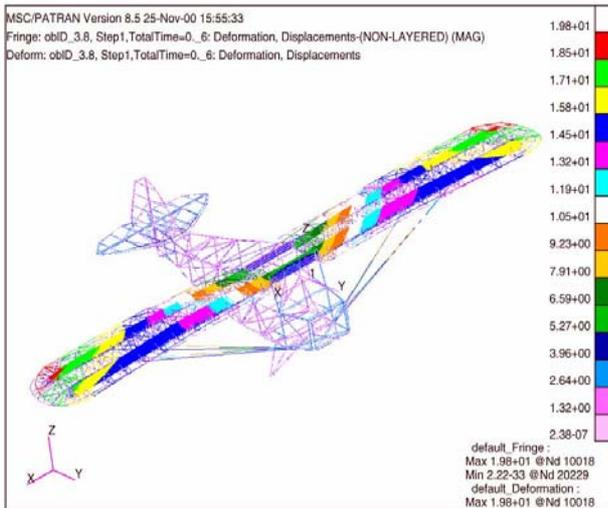
Fig 4. Displacement magnitudes caused by overload in point D
