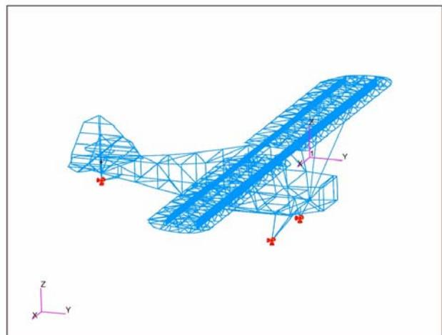
Fig 3. The numerical model of light airplane structure
