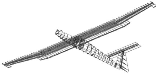
Fig 8. The sailplane geometry (covering is not shown)
