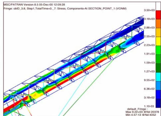
Fig 6. Effective stress in main spar (von Misses). Tension of bottom strips at level of 350[MPa]
