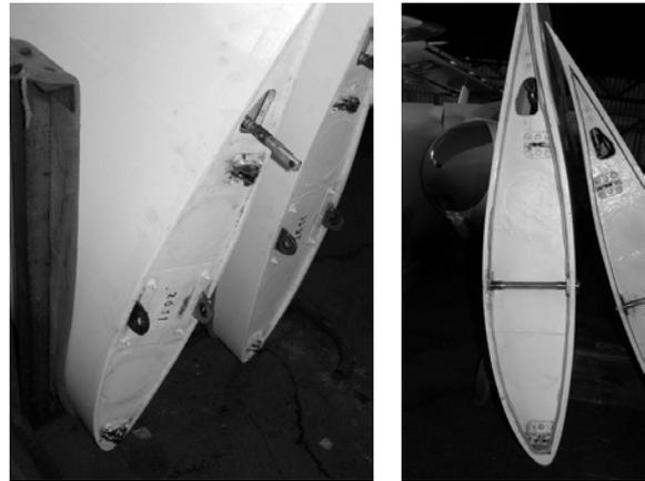
Fig 11. Joints between wing segments. Centre-wing left, wing tip right
