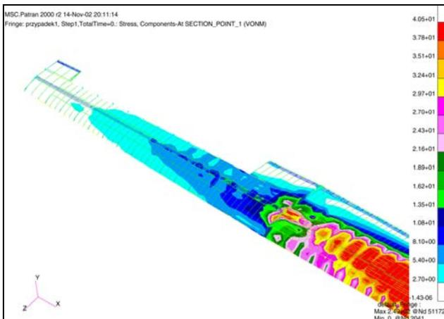
Fig 10. Effective stress concentration (von Mises) around wingtip and centre wing connection
