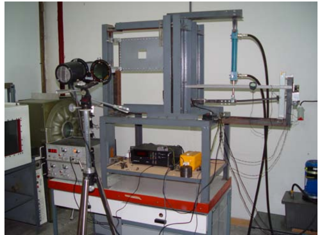
Fig 13. Station for the fatigue test
