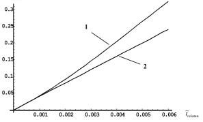
Fig 2. Dependencies of tension change (in relative units) in local area of heterogeneity with constant speed of specimen loading:  $1 - \kappa = 0,4$ ;  $2 - \kappa = 0$ . For both graphs  $\alpha = 40$ , b = 15
