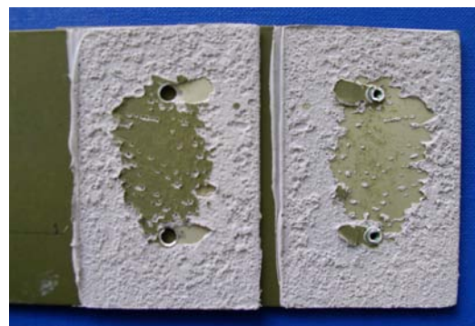
Fig 6. Example failure of adhesive layer
