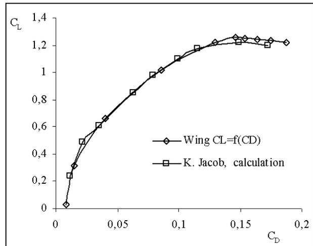
**Fig 11.** Lift-drag characteristics for a NACA 4415 not tapered swept wing (20 deg.) with AR=6.2 at Re=2.1x10<sup>6</sup>. Experimental airfoil results were used as 2D section data
