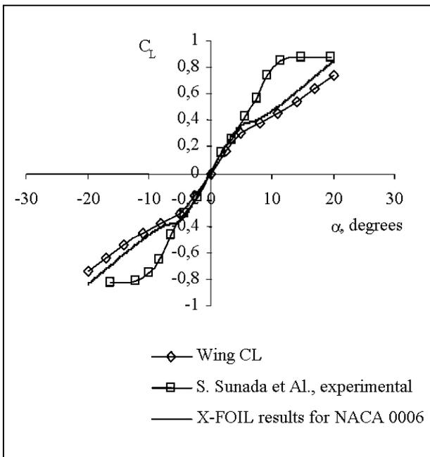
**Fig 6.** Lift coefficient of NACA 0006 rectangular wing with AR=7.25 at Re=4000. X-FOIL calculation results were used as 2D section data
