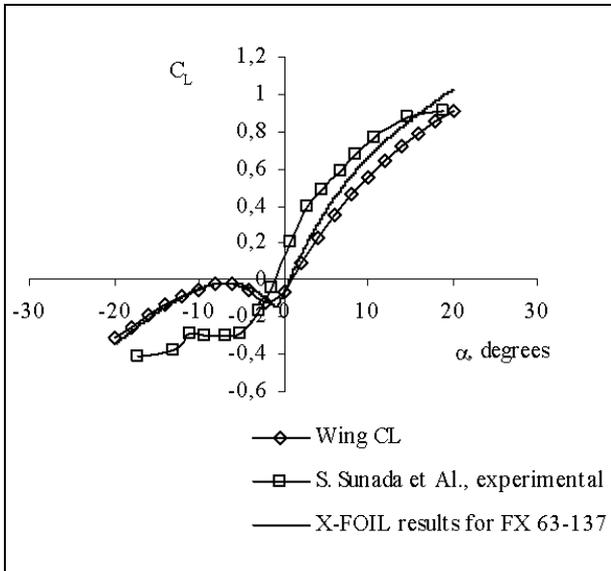
**Fig 5.** Lift coefficient of FX 63-137 rectangular wing AR=7.25 at Re=4000. X-FOIL calculation results were used as 2D section data
