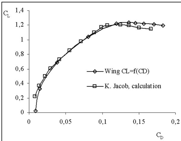
**Fig 10.** Lift-drag characteristics for a NACA 4415 rectangular wing with AR=6.2 at Re=2.1x10<sup>6</sup>. Experimental results were used as 2D section data
