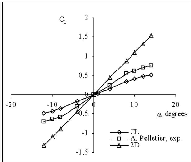
**Fig 3.** Lift coefficient of a rectangular wing of aspect ratio 3 at  $Re=140000$ . For calculation, section experimental results were used
