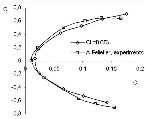
**Fig 2.** Lift-drag characteristics for a flat plate rectangular wing with aspect ratio 3 at  $Re=80000$ . For calculation, section experimental results were used
