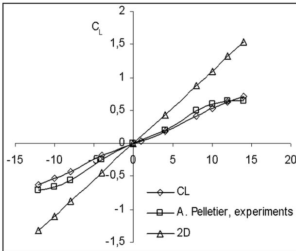
**Fig 1.** Lift coefficient of a flat plate rectangular wing of aspect ratio 3, at  $Re=80000$ . For calculation, section experimental results were used
