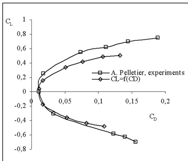
**Fig 4.** Lift-drag characteristics for a rectangular wing with aspect ratio 3 at  $Re=140000$ . For calculation, section experimental results were used
