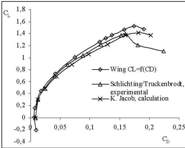
**Fig 9.** Lift-drag characteristics for a NACA 2412 rectangular wing with AR=5 at Re=2.7x10<sup>6</sup>. X-FOIL calculation results were used as 2D section data
