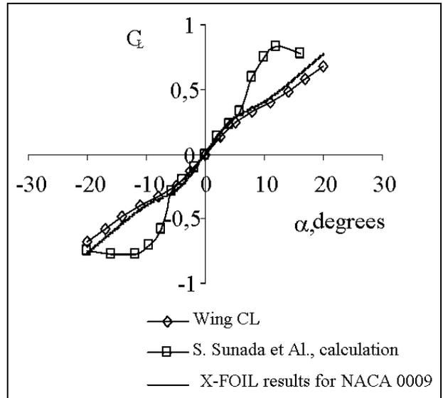
**Fig 7.** Lift coefficient of NACA 0009 rectangular wing with AR=7,25 at Re=4000. X-FOIL calculation results were used as 2D section data
