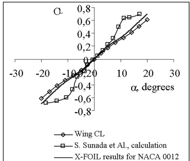
**Fig 8.** Lift coefficient of NACA 0012 rectangular wing with AR=7.25 at Re=4000. X-FOIL calculation results were used as 2D section data
