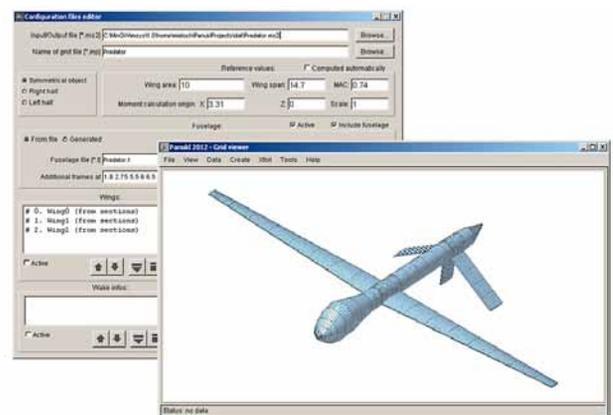
Fig. 1. The GUI of the MS2editor (Panukl pre-processor)
