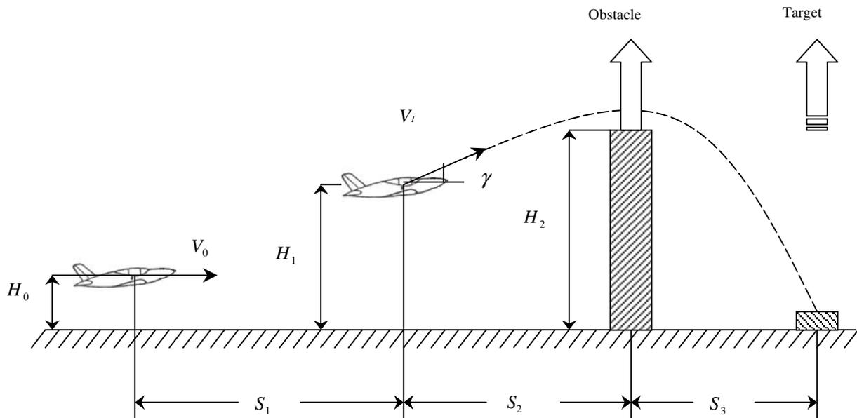
Fig 1. Illustration of problem. The interrupted line is the trajectory of the bomb after it has been dropped
