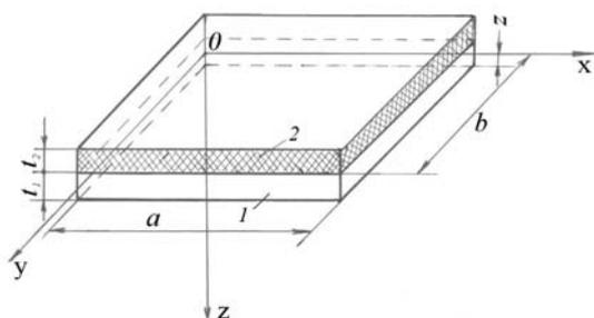
Fig 1. Two-layer plate: 1) supporting metal layer, 2) plastic coating
