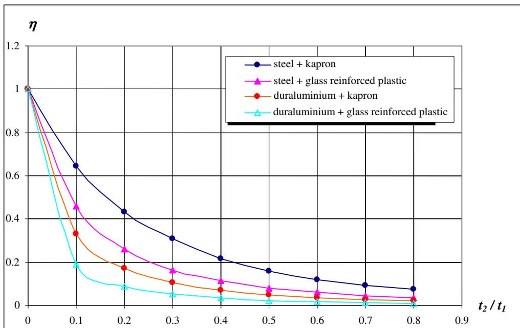
**Fig 2.** Effect of thickness of coating on level of vibration
