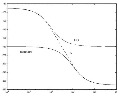
**Fig 7.** Bode diagrams for systems pilot-airplane in the heading channel for classical plane and for heading oriented control if PD-type or P-type heading rate regulator used
