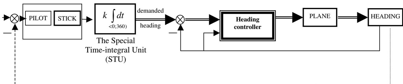
Fig 8. The schematic of the Heading Rate Control Heading Keep (HRCHK) algorithm
