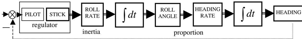
Fig 4. Pilot-aircraft system in heading channel
