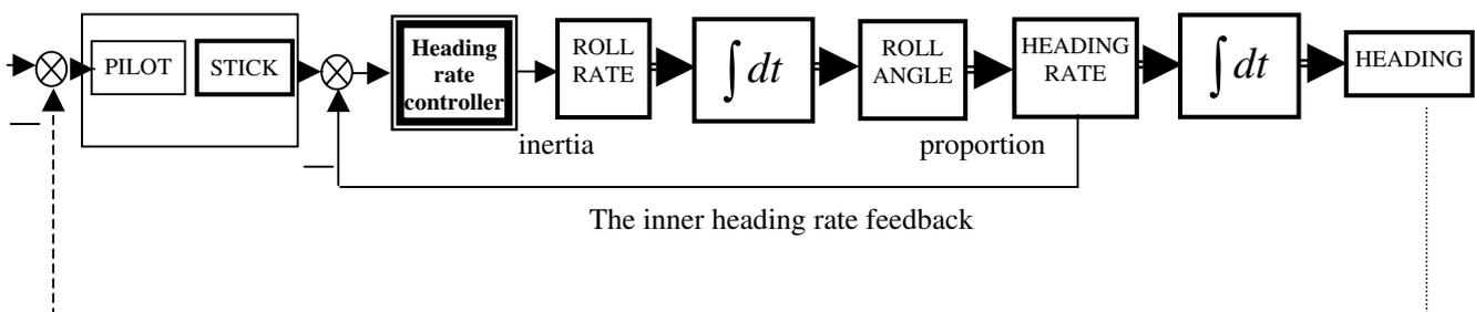
Fig 6. The schematic of the pilot-airplane system in the heading-oriented case of the control
