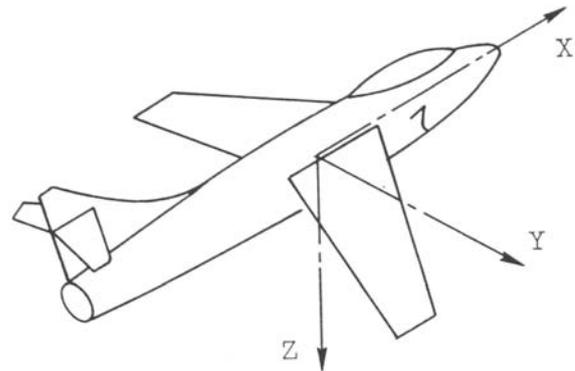
Fig 2. The airplane axis system with its origin located in plane's center of gravity
