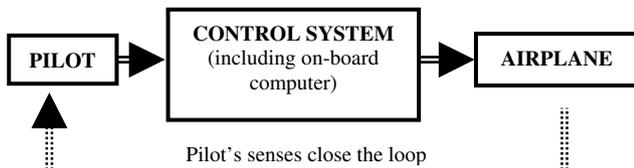
Fig 1. The schematic of the manual computer-aided control system
