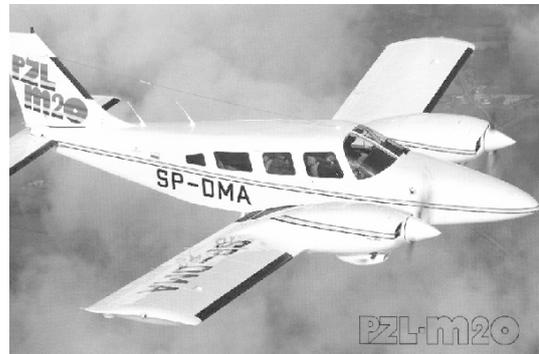
**Fig 1.** PZL-110 “Mewa” – test platform and demonstrator of digital autopilot APC-1 (1988–1990)
