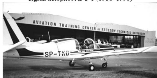
**Fig 2.** PZL-110 “Koliber” – demonstrator of UAV control and navigation system APC-04 (1996–1999), test platform of SPS-1/A fly-by-wire system for GA (2001–2006)
