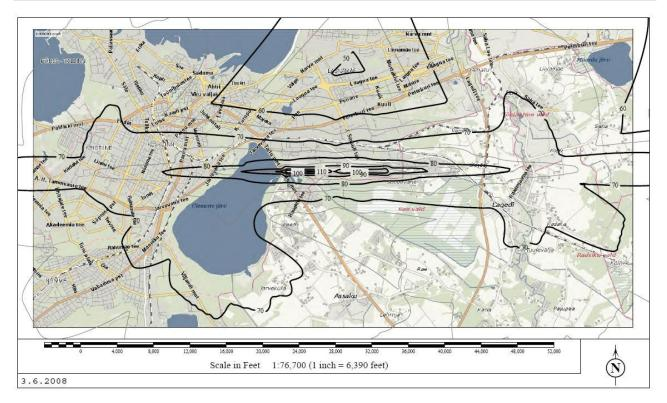
Fig 7. Tallinn Airport. Noise map according to Directive 2002/49/EC. LAmax (7-23) noise contours. 2006 average traffic
