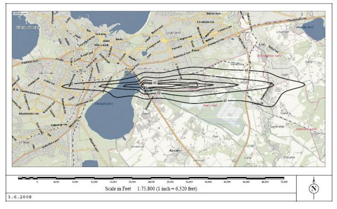
Fig 5. Tallinn Airport. Noise map according to Directive 2002/49/EC. Lnight (23-07) noise contours. 2006 average traffic
