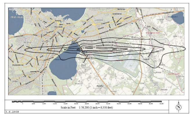
Fig 4. Tallinn Airport. Noise map according to Directive 2002/49/EC. Lden noise contours. 2006 average traffic
