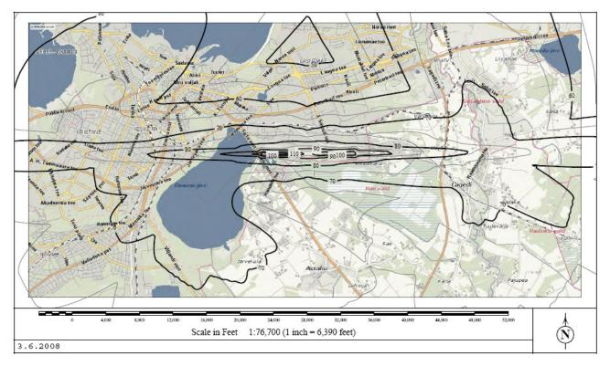
Fig 8. Tallinn Airport. Noise map according to Directive 2002/49/EC. LAmax (23-7) noise contours. 2006 average traffic
