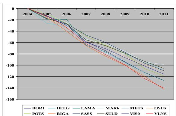
**Fig. 4.** The displacements of coordinate X of the stations (mm)
