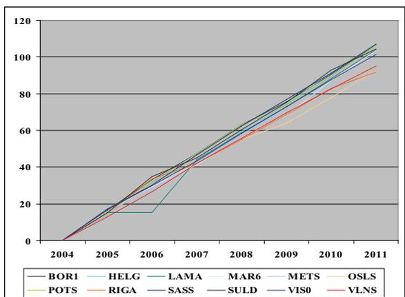
**Fig. 5.** The displacements of coordinate Y of the stations (mm)
