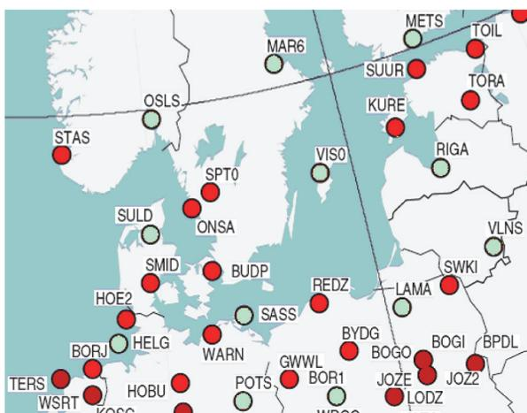
Fig. 3. A detail of a map of the EPN network (The green points – the stations of the EUREF GPS network used in the research, the red points – the stations of the EUREF GPS network not used in the research) (EUREF.. 2011)
