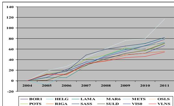
**Fig. 6.** The displacements of coordinate Z of the stations (mm)
