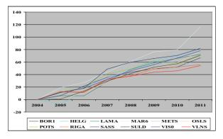
Fig. 6. The displacements of coordinate Z of the stations (mm)
