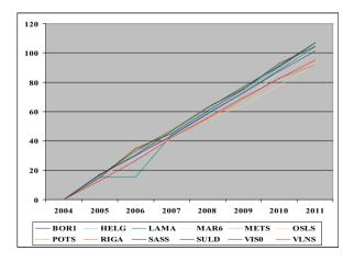
Fig. 4. The displacements of coordinate X of the stations (mm)
