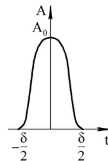
Fig. 1. Form of disturbance impulse during the destruction of composite material
