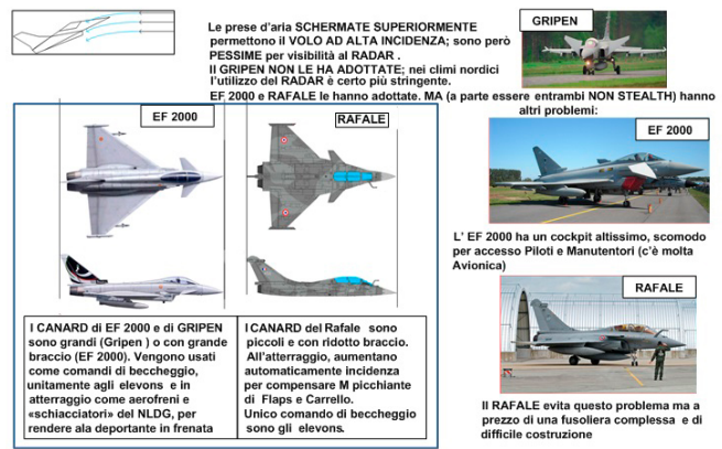
Fig. 9. Analysis of dissimilarities of EF 2000, Rafale, and Gripen
