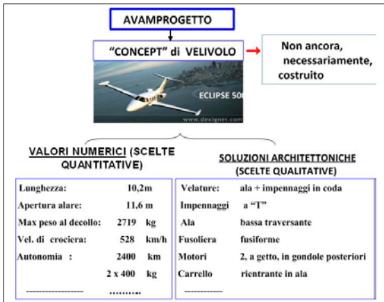
Fig. 2. Architectural characteristics of an aircraft
