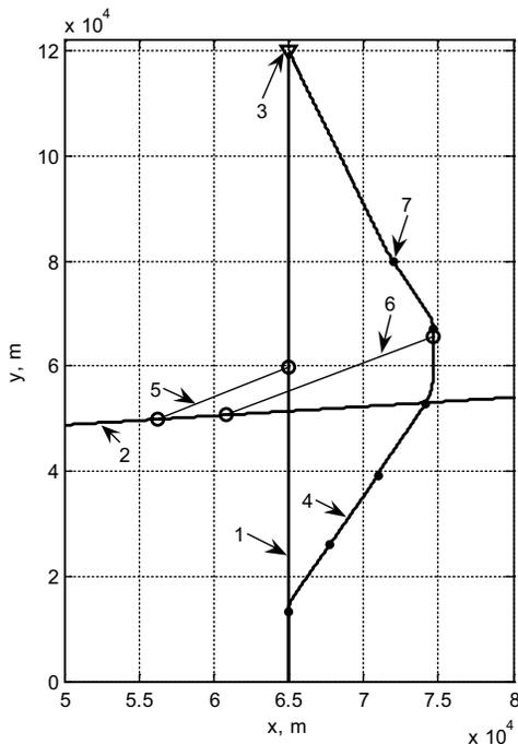
Fig. 4. Aircraft flight trajectories when resolving the conflict situation: 1 – planned flight trajectory of Aircraft 1; 2 – planned flight trajectory of Aircraft 2; 3 – check point; 4 – optimal conflict-free flight trajectory of aircraft 1; 5 – the minimum distance between two aircraft when detecting the conflict; 6 – the minimum distance between two aircraft when resolving the conflict; 7 – states at different stages
