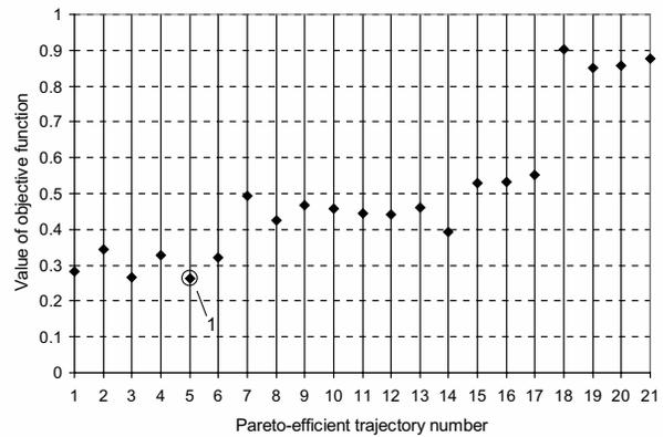
Fig. 3. The value of the objective function,  $\max_{T \in D_w} \sum_{i=1}^3 w_i c_i(T)$ : 1 – function minimum
