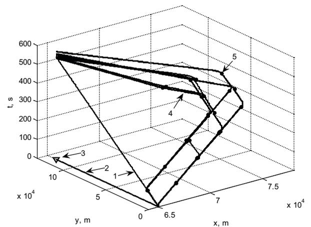
Fig. 1. The set of Pareto-effective flight trajectories of Aircraft 1 in the space-time coordinate system: 1 – planned trajectory; 2 – planned trajectory in the airspace coordinate system; 3 – check point on the route; 4 – Pareto-effective conflict free trajectories; 5 – states at different stages
