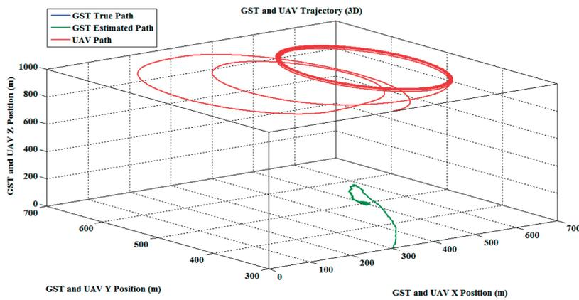
Fig. 5. UAV trajectory circles over a GST (3D)
