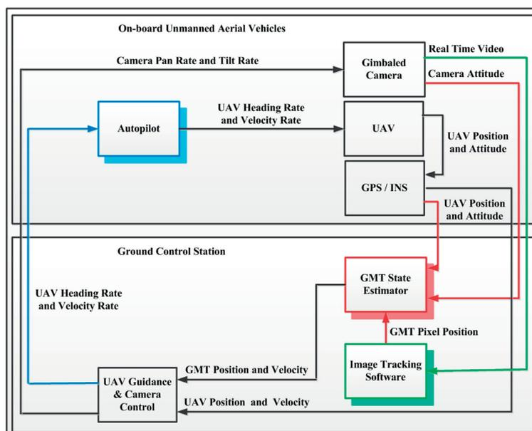
Fig. 1. Architecture of an existing AVTS (an AVTS controlled by a GCS)
