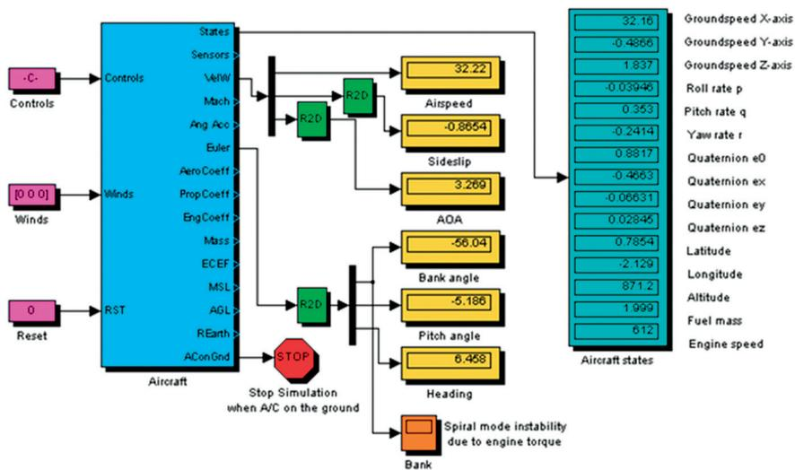
Fig. 3. Simulation – an open loop Simulink model
