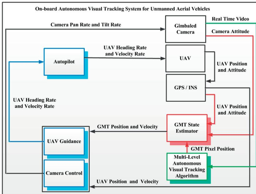
Fig. 2. Proposed architecture for an on-board AVTS (AVTS controlled by the on-board multi-level autonomous visual tracking algorithm)
