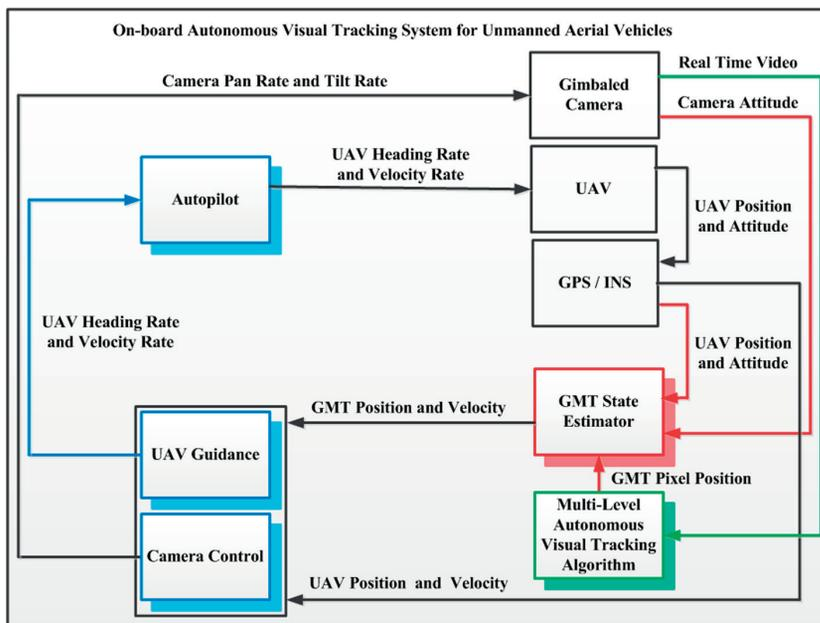
Fig. 2. Proposed architecture for an on-board AVTS (AVTS controlled by the on-board multi-level autonomous visual tracking algorithm)
