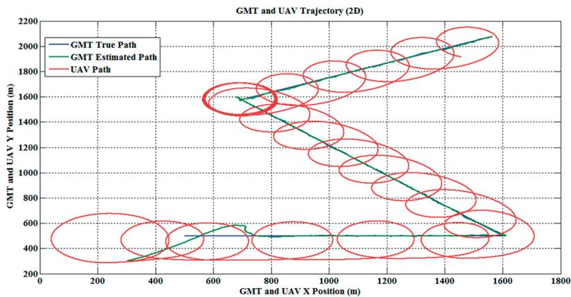
Fig. 6. UAV trajectory circles over a GMT (2D)
