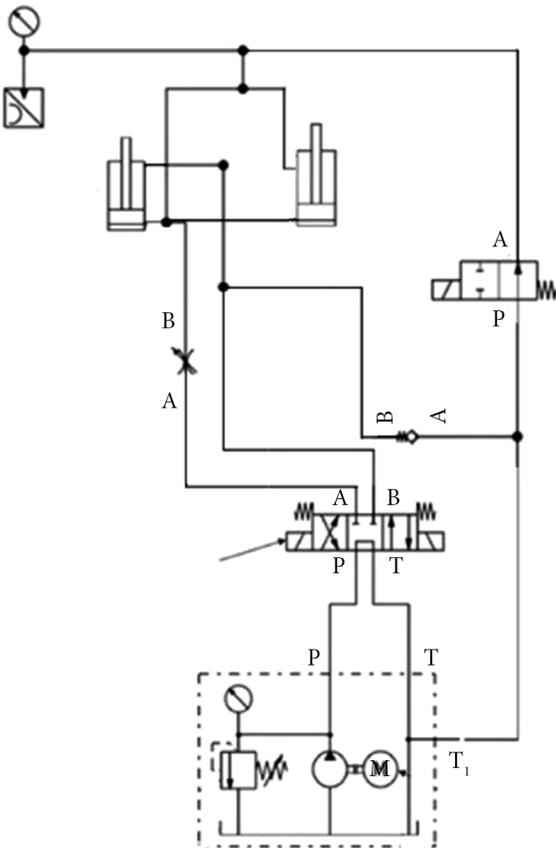
Fig. 7. Hydraulic circuit of the torque generator system
