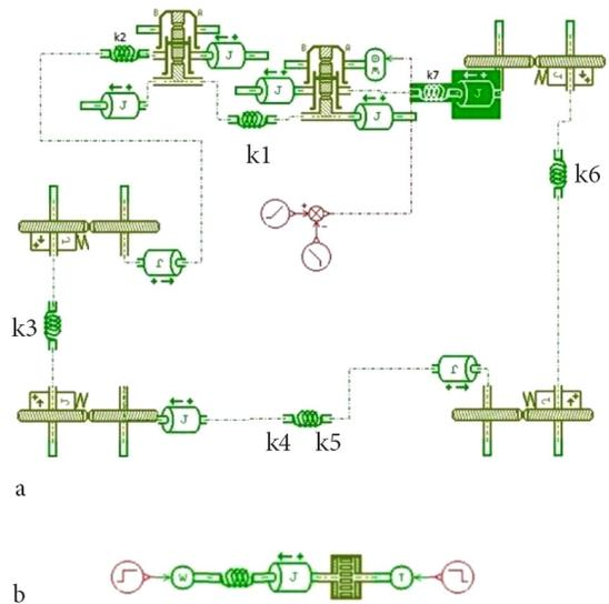
Fig. 11. Modelling results: a) simulated model of the system in AMESIM; b) simplified open-loop model of the system in AMESIM
