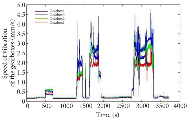
Fig. 14. Vibrations of the gearboxes during the test versus time
