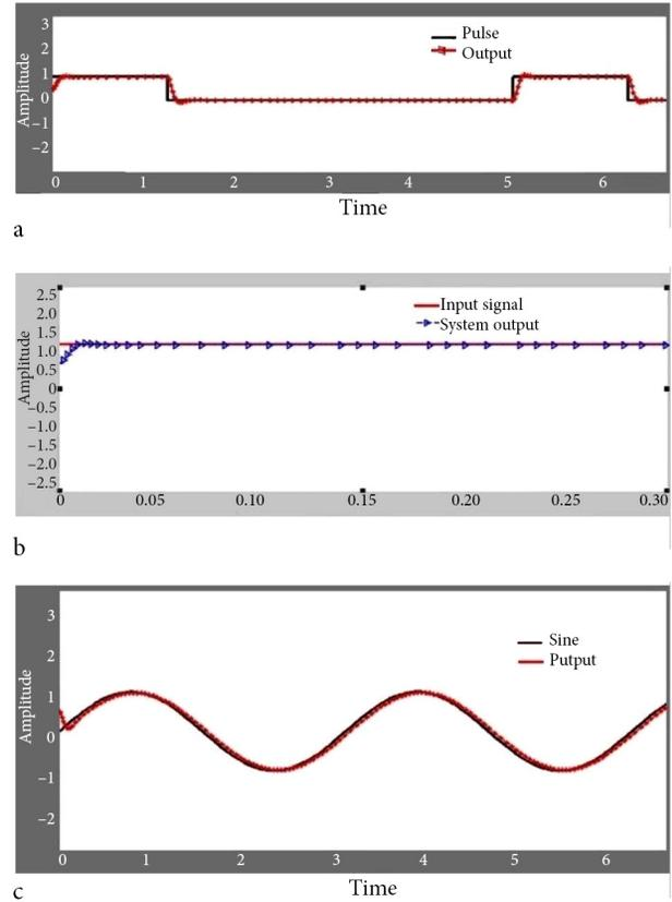
Fig. 9. Responses: a) response of the system to a pulse signal; b) response of the system to a step signal; c) response of the system to a sine signal
