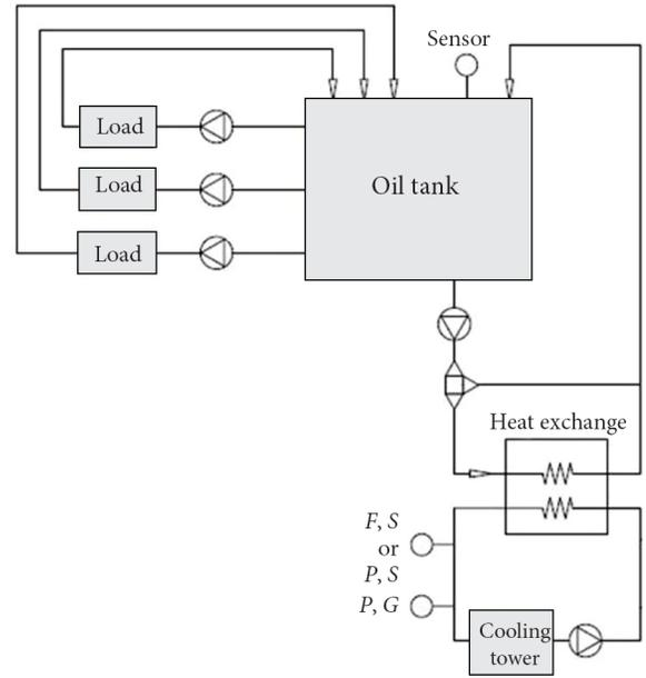
Fig. 10. Circuit of the oil cooling system of the torque generator gearbox
