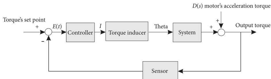
Fig. 8. Loop of the torque generator system's control
