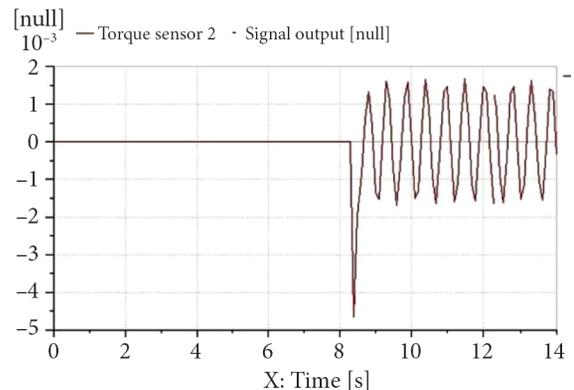
Fig. 12. Torque generated in the model of the system due to a ramp torsion input
