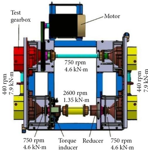
Fig. 1. The test rig with nominal speeds and torques
