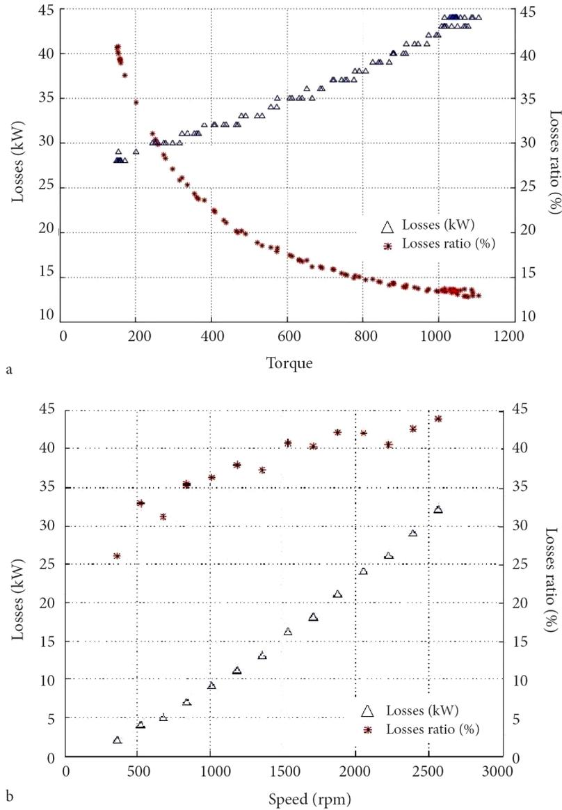
Fig. 15. a) Losses and loss ratio of the system with constant 3000 rpm speed and variable torque; b) losses and loss ratio of the system with constant 150 N.m torque and variable speed
