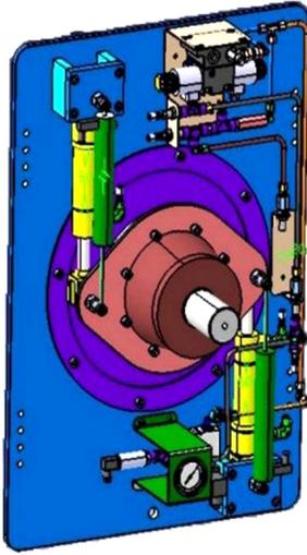
Fig. 6. System of torque generator
