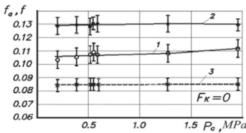
Fig. 3. Dependence of the adhesion component of the friction factor  $f_a$  (curves 1, 2) and the friction factor  $f$  after the micro running-in (curve 3) on contour pressure  $p_C$  for surfaces without micro grooves
