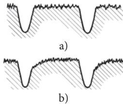
Fig. 11. Wear of the edge of a micro groove: a) before operation; b) after 1500 hours of operation
