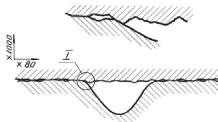
Fig. 10. The engagement of micro asperity projections with the edge of a micro groove in sliding friction
