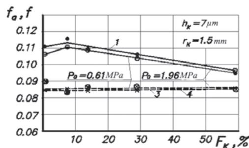
Fig. 5. Dependence of the adhesion component of the friction factor  $f_a$  (curves 1, 2) and the friction factor  $f$  after the micro running-in (curves 3, 4) on the relative area of micro grooves  $F_K$
