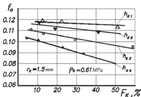
Fig. 6. Dependence of the adhesion component of the friction factor  $f_a$  on the relative area of micro grooves  $F_K$  at a depth of micro grooves  $h_K$ :  $h_{K1} = 20 \mu\text{m}$ ;  $h_{K2} = 11 \mu\text{m}$ ;  $h_{K3} = 7 \mu\text{m}$ ;  $h_{K4} = 3 \mu\text{m}$
