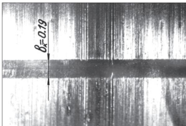
Fig. 14. Traces of penetration of micro asperity projections into the edges of micro grooves, which formed as a result of a micro seizure ( $h_k = 3 \mu\text{m}$ ,  $r_k = 1.5 \text{ mm}$ )
