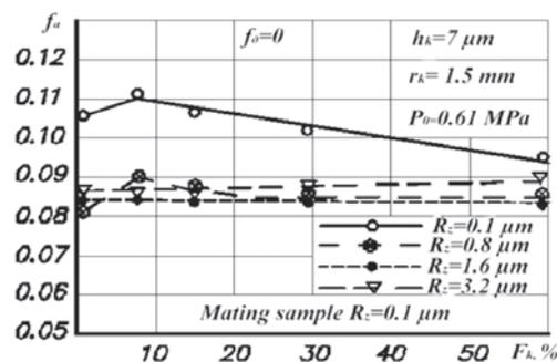
Fig. 9. Dependence of the adhesion component of the friction factor  $f_a$  on the roughness  $R_z$  of the sample carrying surface
