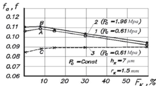
Fig. 4. Dependence of the adhesion component of the friction factor  $f_a$  (curves 1, 2) and the friction factor  $f$  after the micro running-in (curve 3) on the relative area of micro grooves  $F_K$  under constant contour pressure  $p_C$
