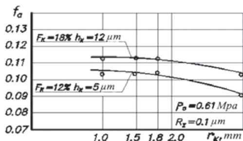
Fig. 7. Dependence of the adhesion component of the friction factor  $f_a$  on the bottom radius of a micro groove  $r_K$
