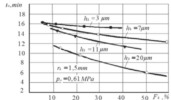
Fig. 13. Dependence of the time of the micro running-in completion  $t_w$  on the relative area of micro grooves  $F_k$
